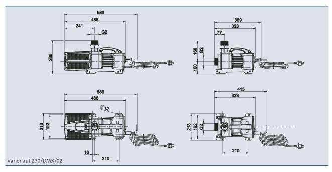
The DMX/RDM controlled Varionaut pump sends back information like temperature, rotation speed, voltage and runtime. The status requests of DMX/RDM allow remote diagnosis and remote maintenance. The Varionaut 270 requires only 380 W and runs with 220-240 V AC voltage at 50 as well as 60 Hz. is A DMX controller, e.g. a WECS II 512 / DMX/02/DMX/02, WECS II 1024 / DMX/02/DMX/02 or WECS II 2048 / DMX/02/DMX/02 server (not included), is required for operating the Varionaut pump.
